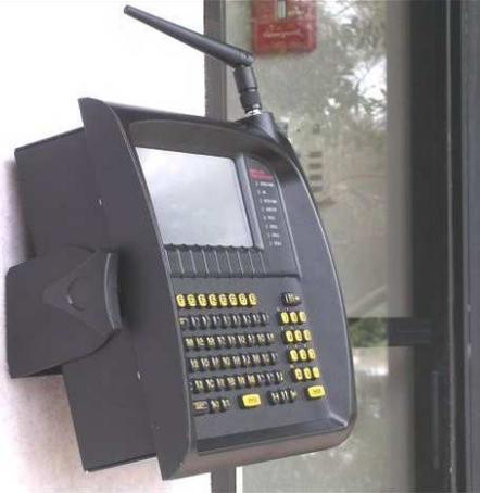
◀ LPA764 provides a convenient way to mount the LANpoint 7 Data Collection Terminal on a wall or other vertical surface.
