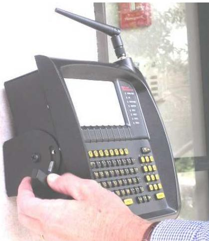
◀ Step 3: insert two (2) bolts & washers in center pivot holes, and insert two (2) handwheels & washers in swivel slot
