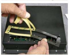
Step 1: Peel & place rubber connector housing seal around connector openings
