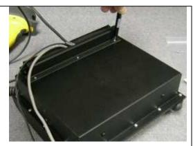
Step 6: Rotate 2<sup>nd</sup> connector housing into place. Adjust in final horizontal position and tighten 3 of the 6 screws
