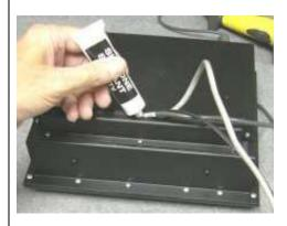
Step 9: Optional: if rubber packing has gaps around cables, use the silicone to seal
